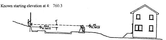
Starting elevation (760.3) + reading on rod (2') = Heigh of Instrument (HI)
